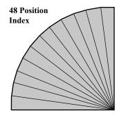
Figure C - Top View, 12 sides at 7.5 degree intervals
