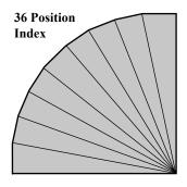
Figure C - Top View, 9 sides at 10 degree intervals
