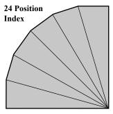
Figure C - Top View, 6 sides at 15 degree intervals
